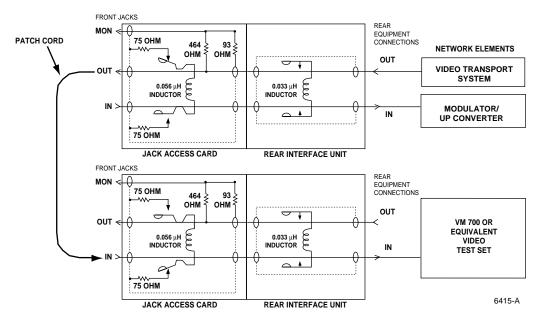
Figure 19. Intrusive Test of Transport Feed
